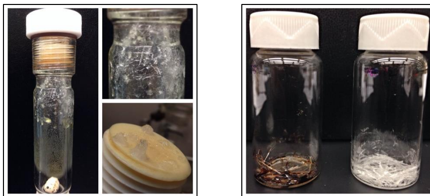
Figure 5. Left: DMT sublimation during reaction. Right: Crude and recrystallized DMT.
